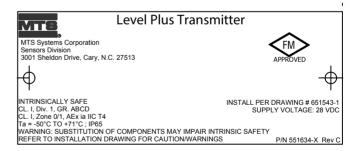
Fig. 14: Intrinsically Safe FM label, Modbus or DDA, Single or Dual Cavity Housing
