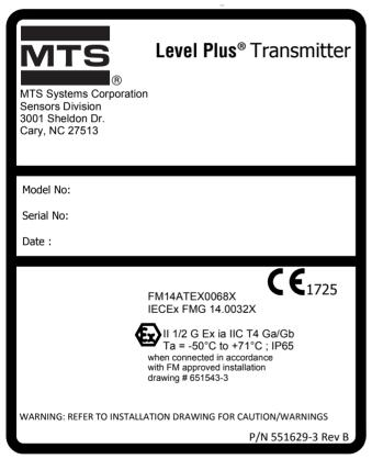
Fig. 47: Intrinsically Safe ATEX/IECEx label, Modbus and DDA, NEMA Housing
