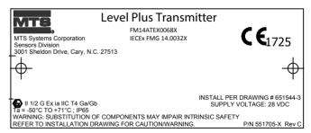
Fig. 50: Intrinsically Safe ATEX/IECEx label, Modbus and DDA, Single and Dual Cavity Housing
