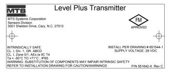
Fig. 15: Intrinsically Safe FM label, HART®, Single or Dual Cavity Housing
