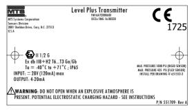
Fig. 56: Flame Proof, ATEX and IECEx label, HART®, Housing Option D, E, G, H, or L
