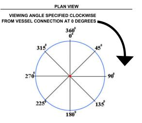
TO SPECIFY THE ASSEMBLY ORIENTATION TWO REFERENCE POINTS MUST BE IDENTIFIED, THE VESSEL CONNECTION AND VIEWING ANGLE. THE VESSEL CONNECTION IS SET AT 0 DEG. THE VIEWING ANGLE IS SET AT ANY DESIRED POSITION WHERE CLEARANCE PERMITS. THE STANDARD VIEWING ANGLE IS 180 DEG FOR ALL GLASS-TRAC GAGE ASSEMBLIES, UNLESS NOTED OTHERWISE. IF A NON-STANDARD VIEWING ANGLE IS REQUIRED, SPECIFY THE VIEWING ANGLE.
