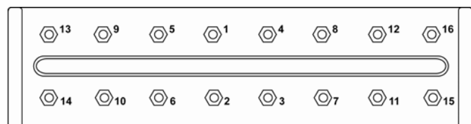
Figure 1—Bolt Tightening Sequence
