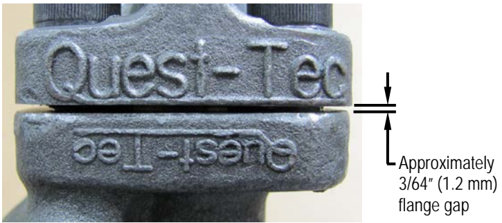
Fig. G-3-A. MODEL SV-1600 VALVE Gap between yoke and valve body flanges will be approximately 3/64" (1.2 mm) when properly tightened.
