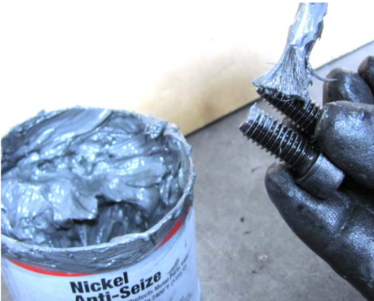
Fig. E-1. Apply nickel-based anti-seize lubricant to the screw threads of the four (4) body/yoke flange cap screws; set screws aside.
