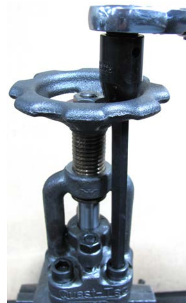
Fig. G-2. Insert a 3/8" straight hex wrench through handwheel openings and in an alternating cross-pattern, tighten screws evenly making 3-4 passes to a final torque of 35 ft.-lbs. (48 Nm).
