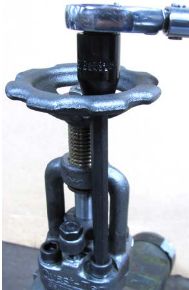
Fig. A-2. Remove cap screws with a 3/8" straight hex wrench inserted through handwheel openings.
