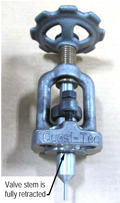
Fig. F-1. Verify that the valve stem is fully retracted to the open position - turn handwheel counter-clockwise until travel limit stop is reached as shown.
