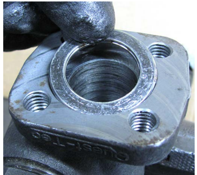
Fig. E-2. Place new spiral-wound gasket into the valve body recess.
