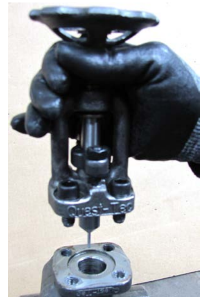
Fig. A-3. Note position of yoke then lift sub-assembly straight outward from valve body.
