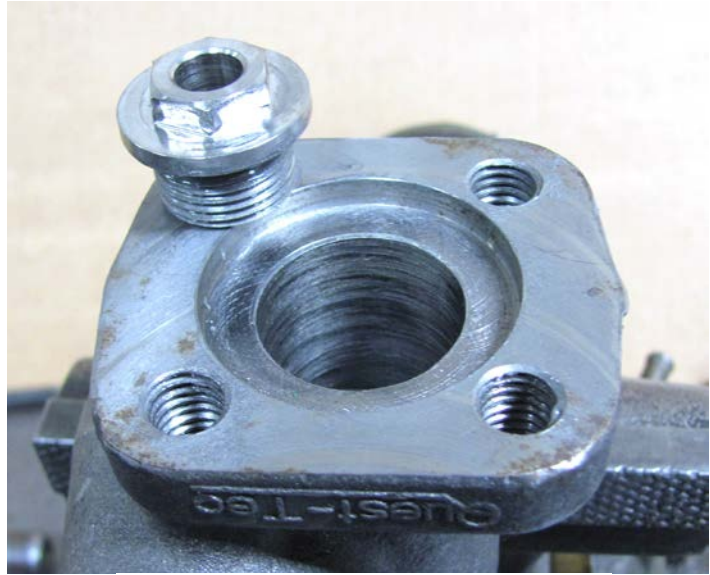
Fig. B-2. Valve seat removed from valve body.
