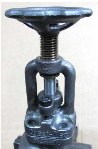
Fig. G-1. Orient the new yoke/stem sub-assembly (relative to the valve body) in the position as was the previously removed (old) sub-assembly.
