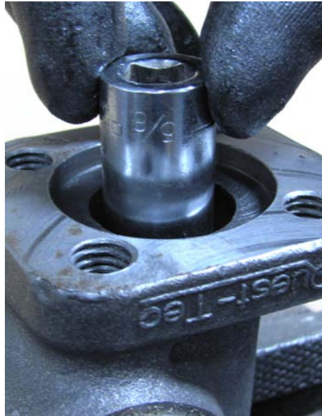
Fig. D-2. Install valve seat & tighten finger-tight using 5/8" socket wrench.
