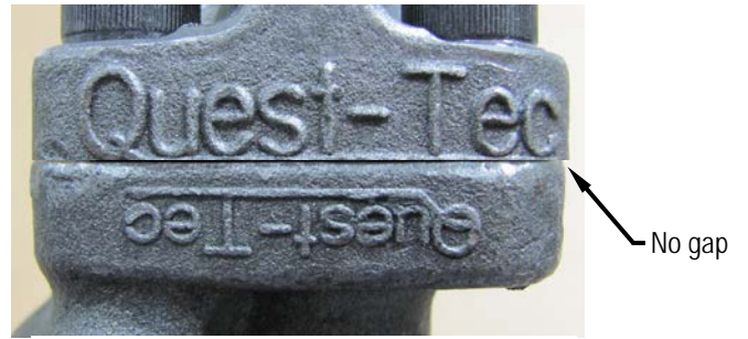
Fig. G-3-B. MODEL SV-1600A VALVE Yoke and valve body flanges shall be made-up metal-to-metal with no gap when properly tightened.
