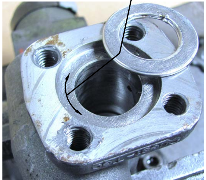
Fig. C-2. Inspect gasket recess in the top of valve body; clean as needed with very fine grit emery cloth or steel wool.
