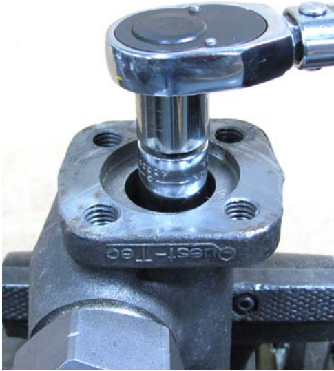
Fig. B-1. Unthread valve seat from valve body bore with a 5/8" socket & ratchet/torque or bar wrench.
