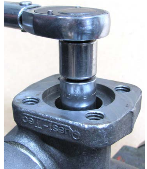
Fig. D-3. Attach wrench to socket and tighten valve seat to 30 ft-lbs. (41 Nm).
