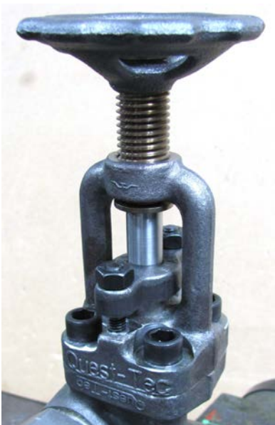
Fig. A-1. Valve body clamped in a vise & valve in the full open position.
